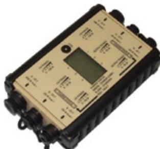
A versatile converter, this intelligent device facilitates compatibility and energy management between a broad range of power sources and numerous end devices as well as rechargeable batteries. **The Power Manager** is extremely practical, allowing users to forgo bringing along scores of different types of batteries and thereby significantly reducing the weight they carry.
